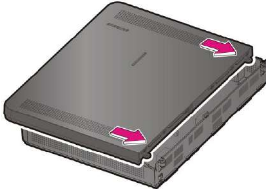
Figure 2.15 Installing the top cover (1)
