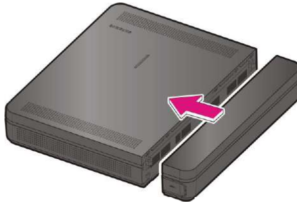
Figure 2.18 Installing the duct cover (1)
