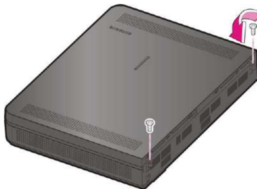
Figure 2.3 Removing the screws
