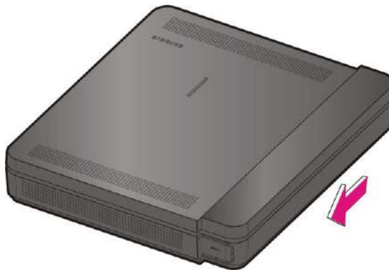
Figure 2.19 Installing the duct cover (2)
