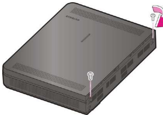
Figure 2.16 Installing the top cover (2)
